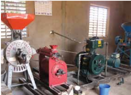
A MFP is an infrastructure of energy that is used for operating different power devices (milling grain and rice, grinding Shea, battery, welding, etc.)
